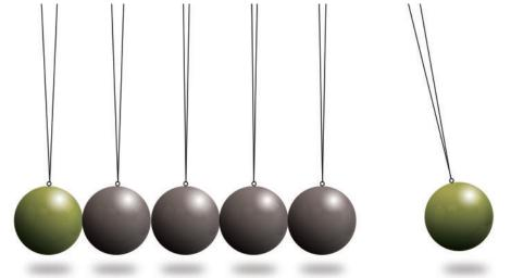
Figure 1. Newton's Cradle. The balls in the middle don't move, but the ball on one end transfers energy through them to make the ball on the other end fly upward. This is how sound is transmitted through solid objects, like walls and doors.
