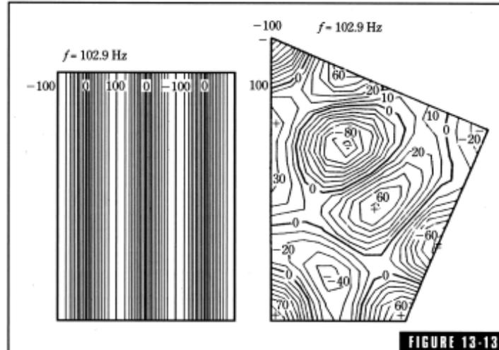
The 3,0 mode of the 5 x 7 meter two-dimensional room of Figs. 13-10 and 13-11, and 13-12 and resulting distortion of the modal pattern when changed to a nonrectangular room of the same area.<sup>8</sup>
