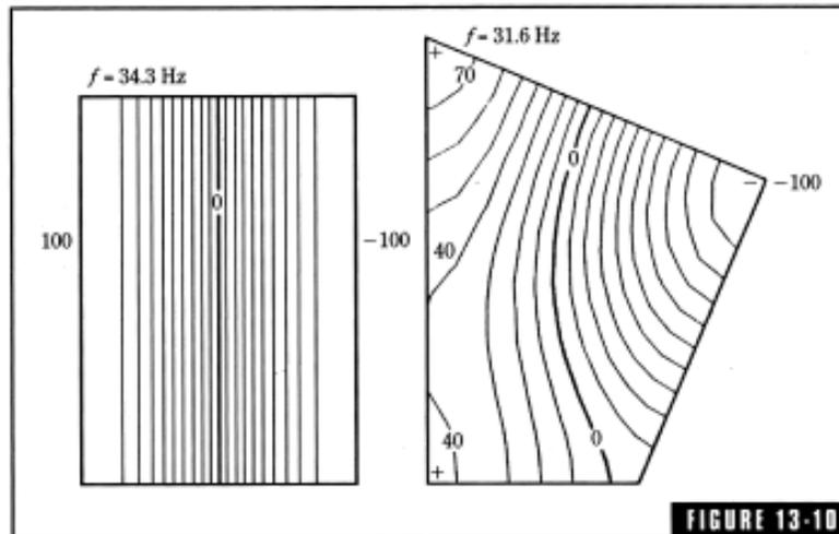
Comparison of the modal pattern for a 5 x 7 meter two-dimensional room and a non-rectangular room of the same area. This sound field of the 1,0 mode is distorted in the nonrectangular room and the frequency of the standing wave is shifted slightly.<sup>8</sup>
